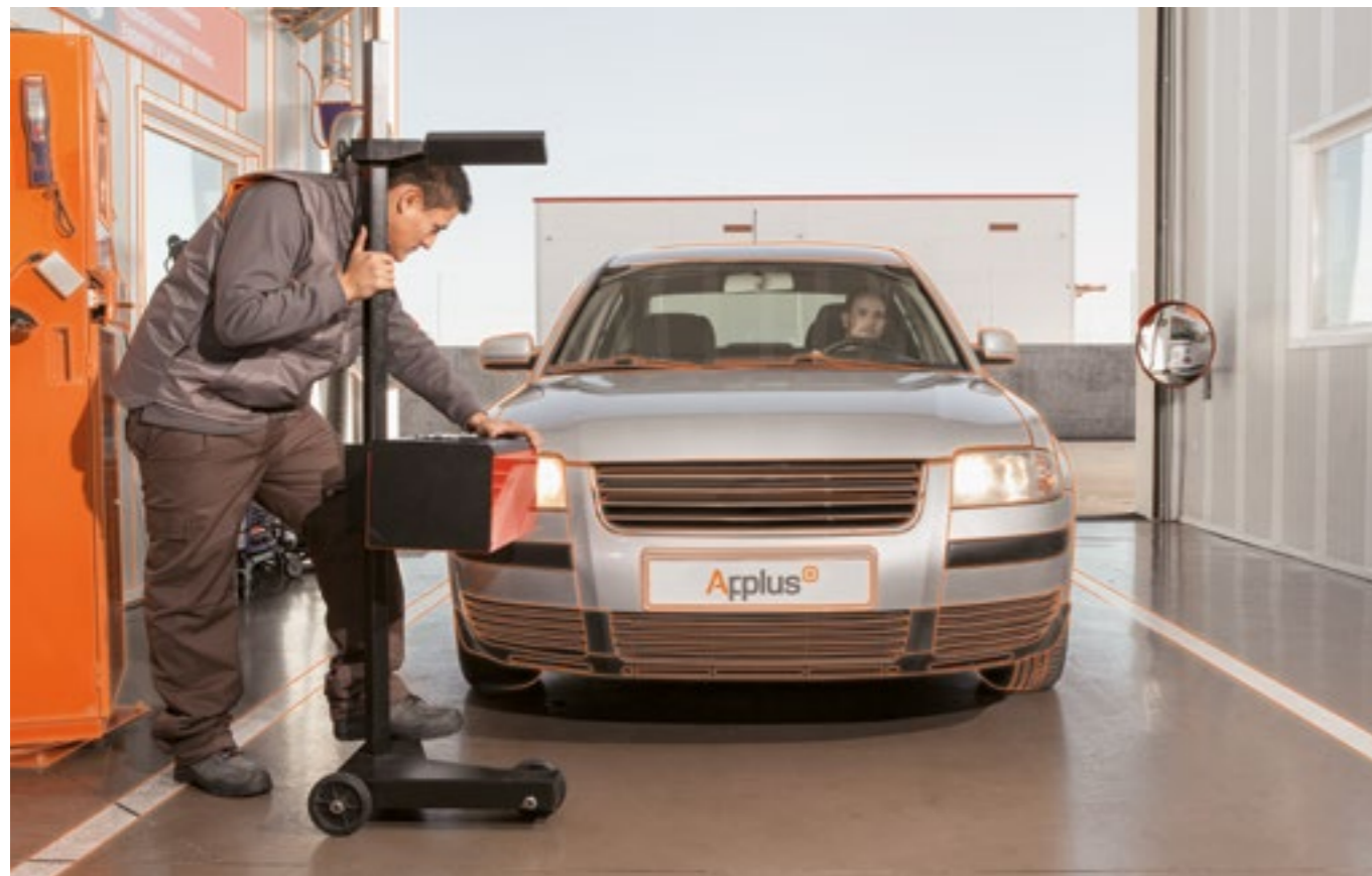
Headlamp alignment testing.
