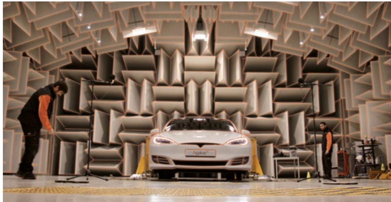
Acoustic testing of an electric vehicle for pedestrian awareness.
