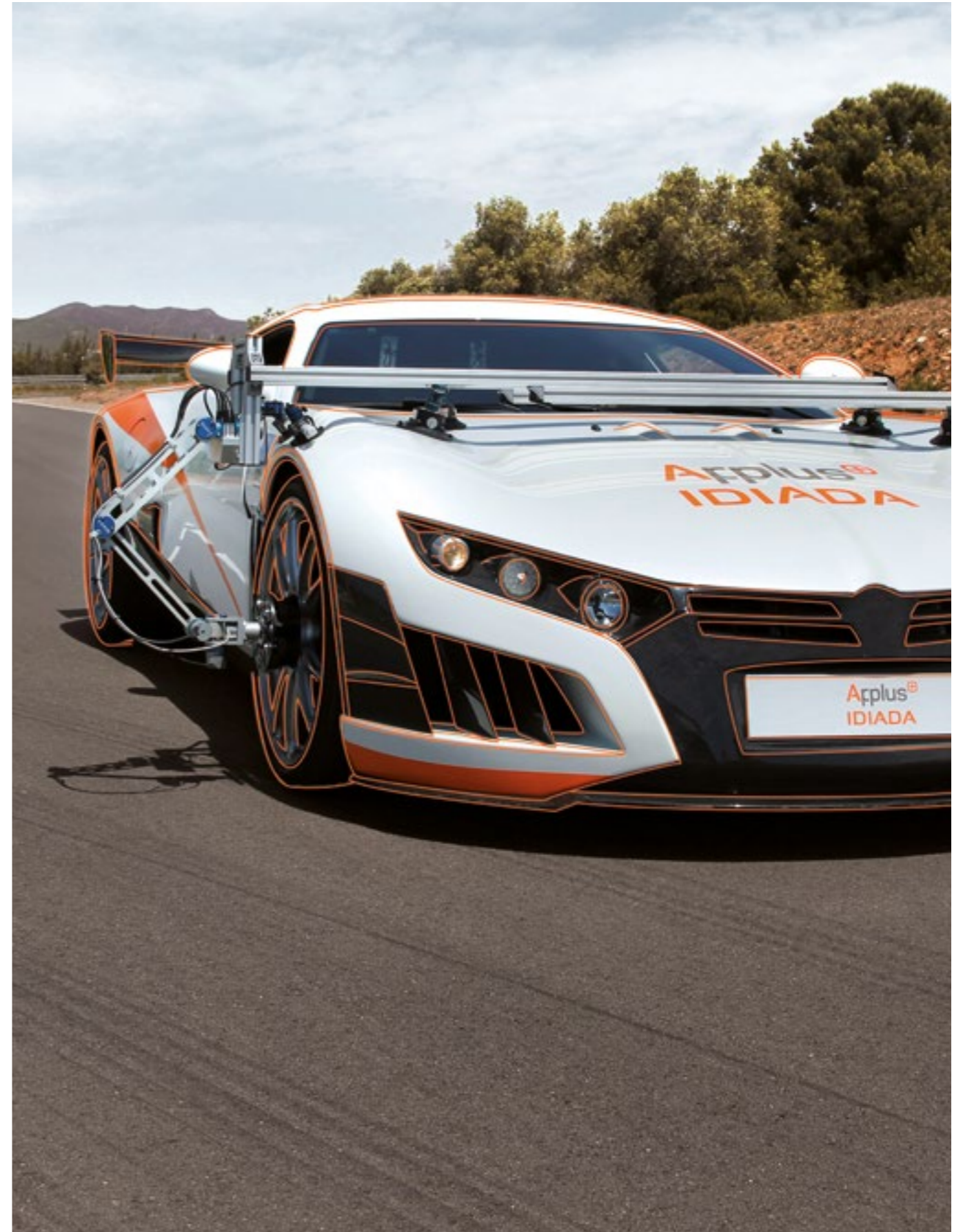
Dynawheel is a wheel position measurement system developed by Applus+ to provide real-time calculation of wheel position in real driving conditions.
