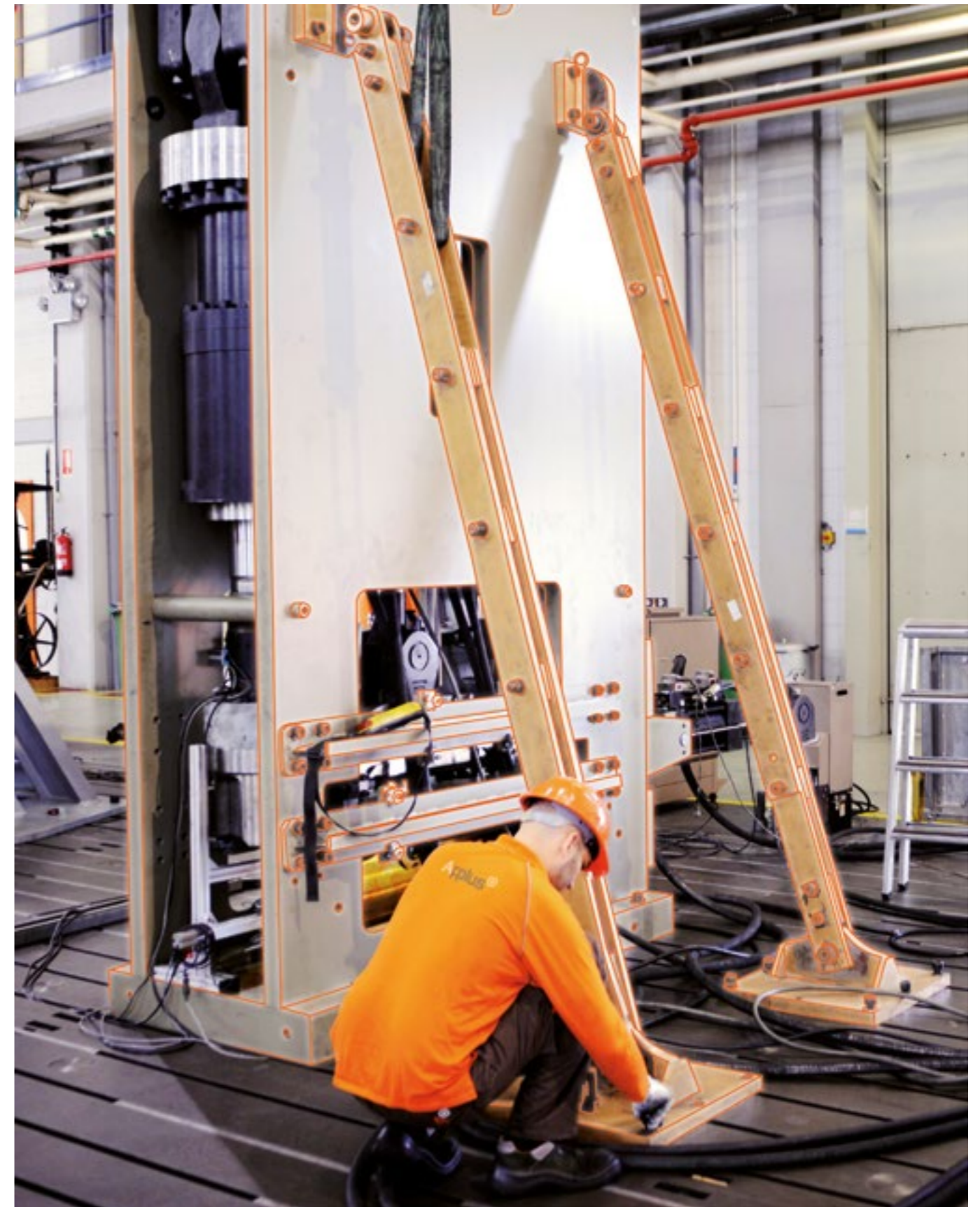
Fatigue test on an aerospace engine mount.
