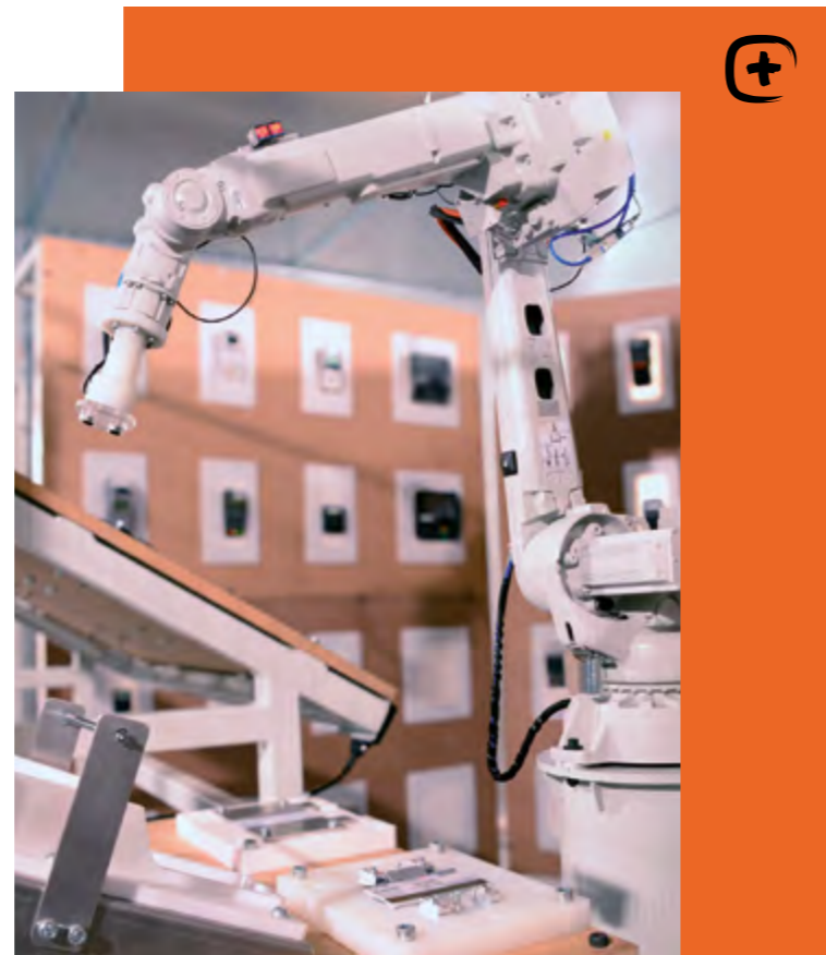
Robotic system: interoperability tests on payment terminals, cards and mobile payment solutions.
