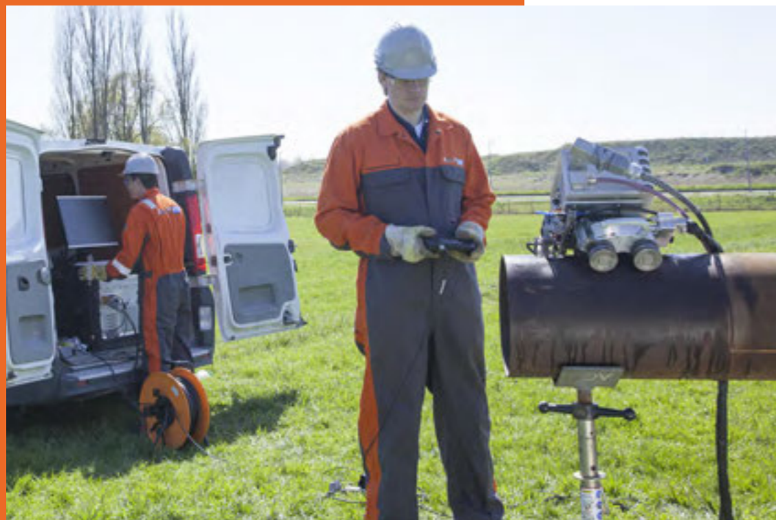
Ultrasonic testing using the RTD IWEX technology
