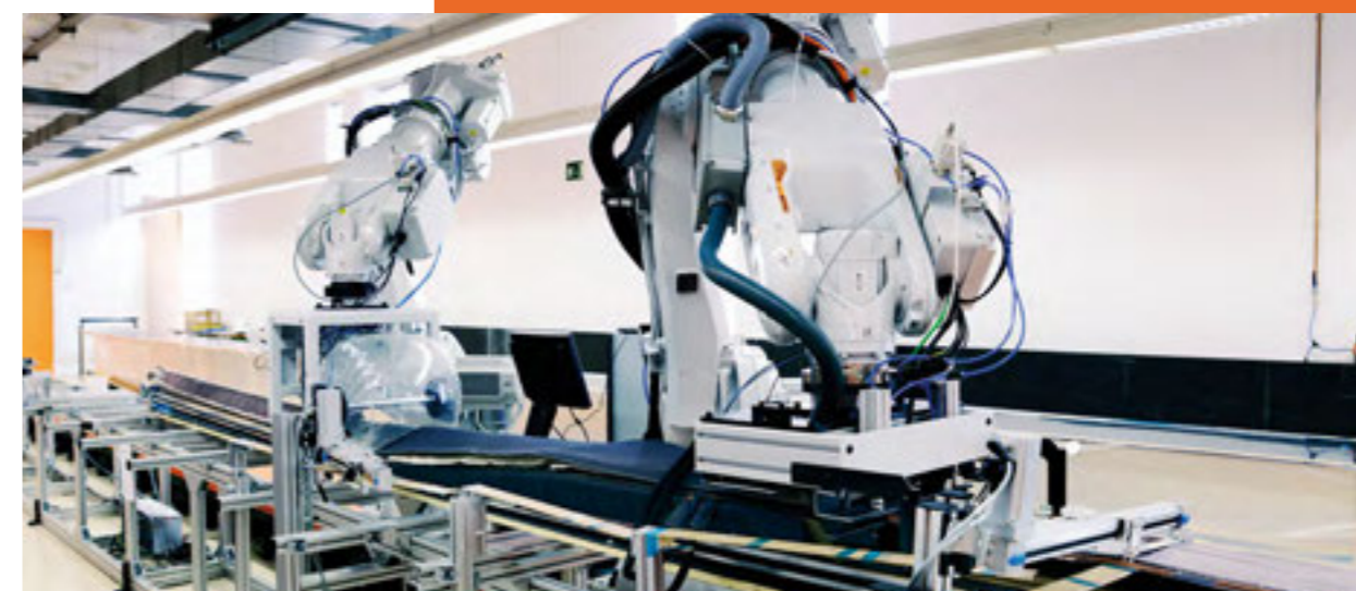
A+ Glide Forming: innovative and proprietary technology for carbon-fibre aircraft stringer manufacturing
